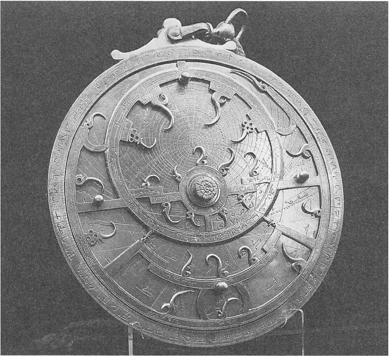
Muslim astronomers perfected the astrolabe to determine astronomical and timekeeping data, as shown above in an 18th-century Persian model.
